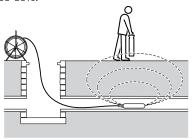
A Sonde radiates a peak field from the center of its axis with ghost signals at each side of the peak. Move the Receiver to one side and then along the axis of the Sonde forwards and backwards to detect the ghost signals.
