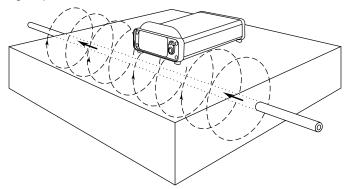
Note: Induction cannot apply a signal to a line below reinforced concrete.
